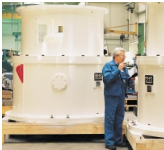
Fig.: 11: BHS Epicyclic Gear Unit, Type RHG, with thrust bearing.
